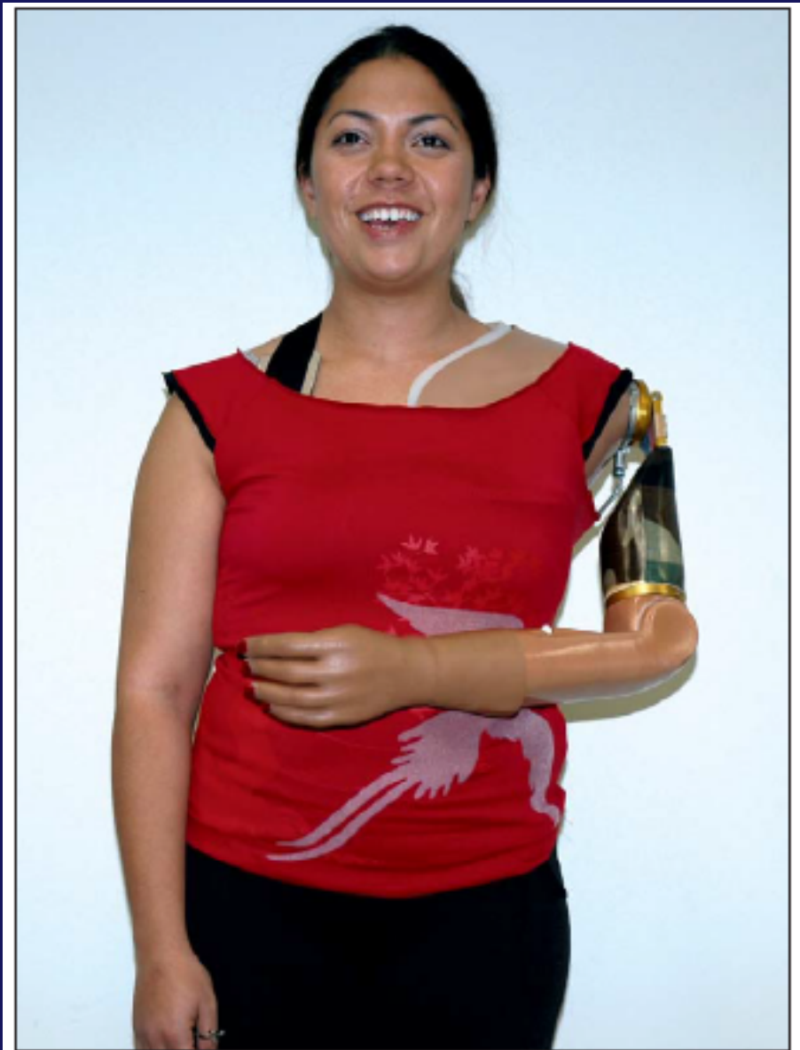
Figure 10: Experimental prosthesis consisting of a motorised elbow, wrist, and hand, with passive shoulder components
